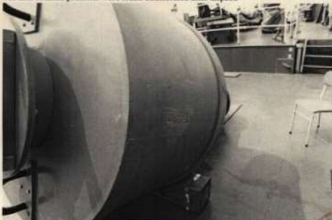
撞击后浮标本体略有划痕，但未发现破裂 A few scratches were found on the buoy but no cracking found after impact.
