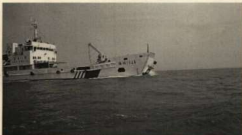
船只以 12 海里/小时速度撞击浮标瞬间 The moment that a ship impact on a buoy at speed of 12 nautical miles per hour.
