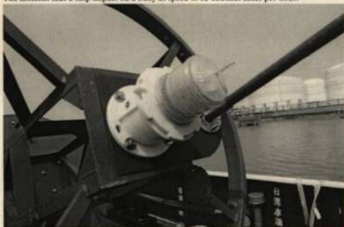
撞击后灯器完好，未发现损坏 The light was found to be in good condition after impact.
