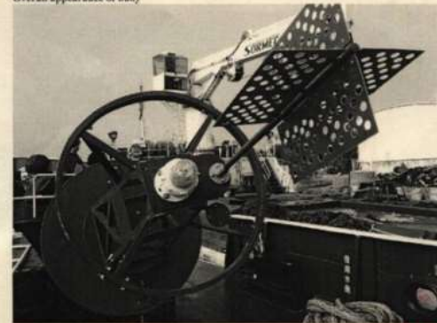
撞击前浮标护圈及灯器 The anti-collision protector and light of buoy.
