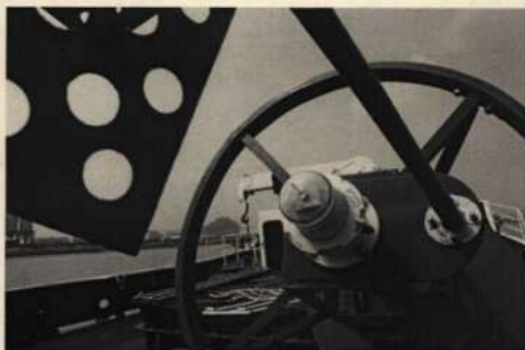
撞击后灯器护圈未发现变形 The anti-collision protector were found undeformed after impact.
